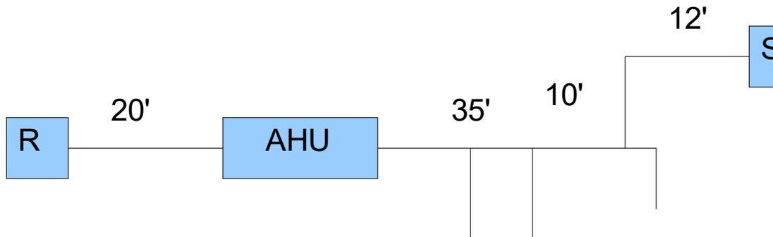
The above illustration shows the longest distance in the duct system is from return R to Outlet S, 77 ft. ( $20+35+10+12 = 77$ ).
